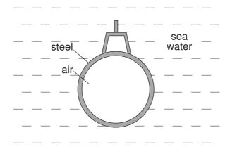
What causes the upthrust on the submarine?
